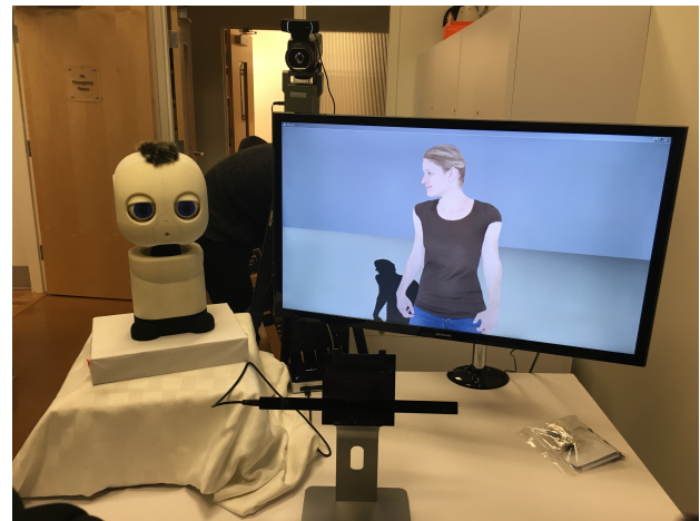
Figure 1. Typical setup of the complete system from the infant’s point of view. Here the robot and avatar (left and right) can be seen with the eyetracker (bottom center) and thermal IR camera (top center).
